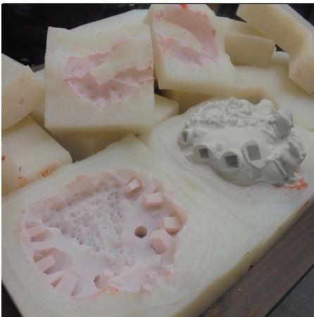
Silicone tooling for the crab. Top: small claw mold. Bottom: two-part crab mold with master pattern pictured.
